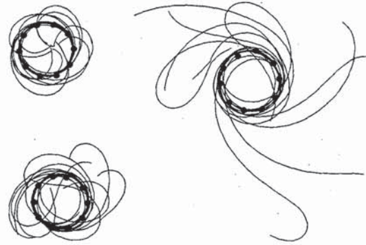
Fig. 4. Circling formation initialization for ten vehicles from three different sets of random initial conditions [3].
